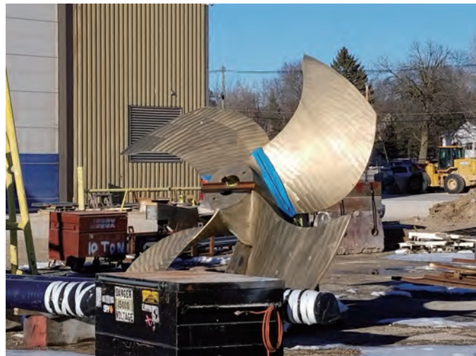
Superston ship propeller repair welded with AMPCO-TRODE® 40.
