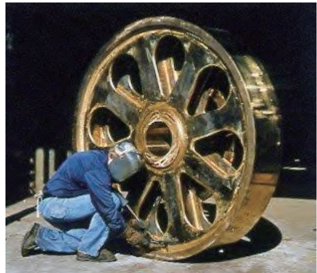
Propulsion Gear: Aluminum Bronze cast & wrought components fabricated into a 4000 lb. propulsion gear for a minesweeper using AMPCO-TRODE® 10. Aluminum Bronze & AMPCO-TRODE® 10 was used for its non-corrosive properties.
