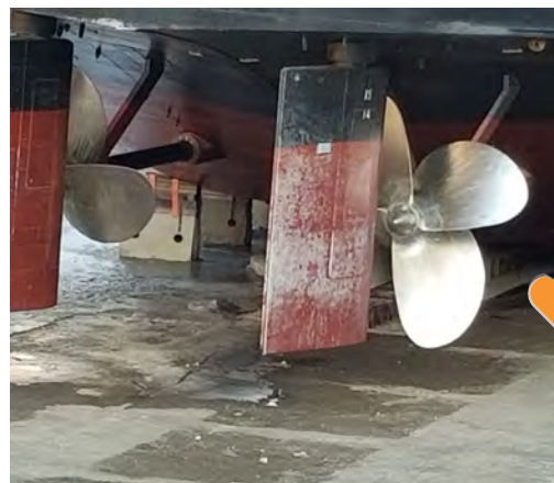
Submarine propulsion unit fabricated with AMPCO-TRODE® 46.
